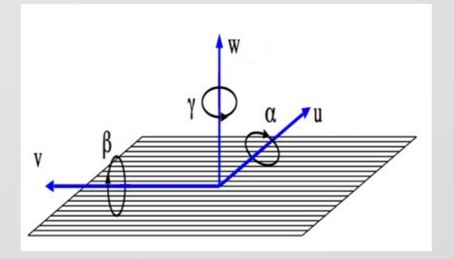
in general, each sensor has 6 alignment parameters ... some are probably insensitive (v,  $\alpha$ ,  $\beta$ ?)
