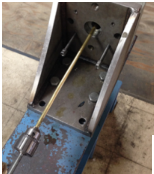
The cable is inserted in a sheath tube, and the sheath is drawn onto the cable to just compress the wires against the spring tube.
