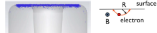
(b) Multipacting electrons near the short plate. (c) Schematic view of the multipaction.
