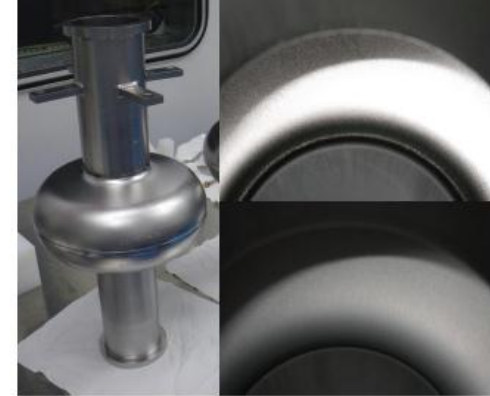
Figure 3: Coated cavity (left); view looking down into cavity before (top right) and after coating (bottom right).
