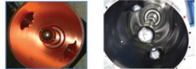
Figure 3: QWR before (left) and after (right) Nb coating.
