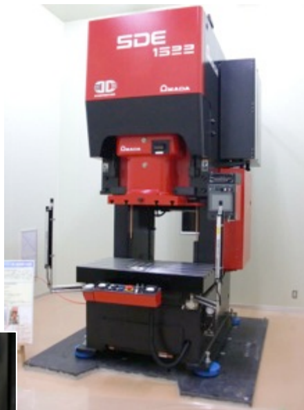
AMADA digital-servo-press SDE1522 150t, 50stroke/min, 225mmstroke
