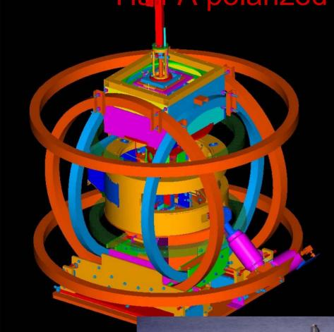
40-cm long Rb-K spinexchange hybrid cell at 10 atm with beam current of 15 μA
