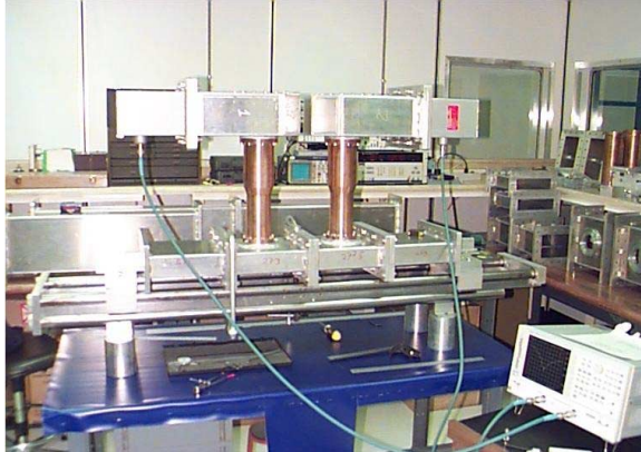
Figure 2: Experimental low-power RF setup for dimensioning the connecting waveguide
