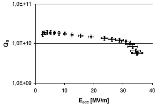
Figure 7: Best performing 9-cell TTF cavity, electropolished.
