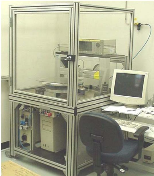
Figure 6: Eddy Current Scanning system used at Jlab for defect scanning of the niobium used for SNS cavities.
