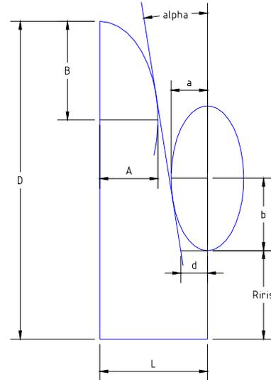
Figure 1: Cross sectional view of an elliptical cavity
