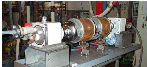
Figure 5: Typical electropolishing set-up as developed at KEK for multi-cell cavities. The cavity is rotated horizontally while acid is circulated through the cavity at an applied voltage of ~ 14 V.
