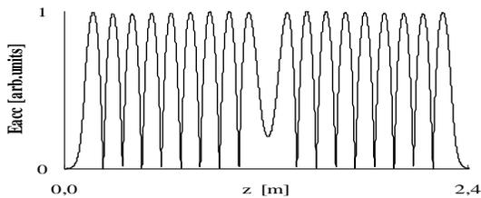
Figure 3: Field profile of the accelerating mode of the super-structure [9].
