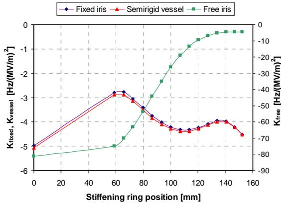
Figure 2: Lorentz force detuning coefficient vs position of stiffening rings (example  $\beta=0.61$  SNS cavity).
