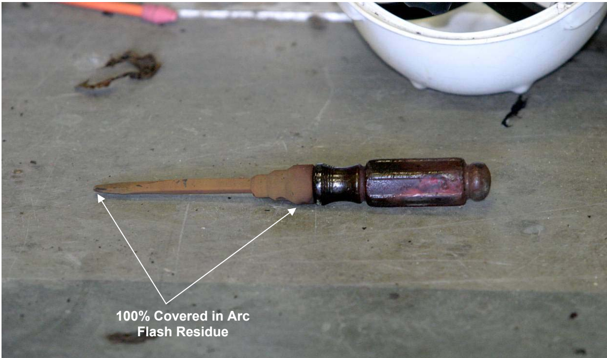
Figure 2-9. Closeup of the screwdriver the Board believes BSE-1 was using when the arc flash occurred
