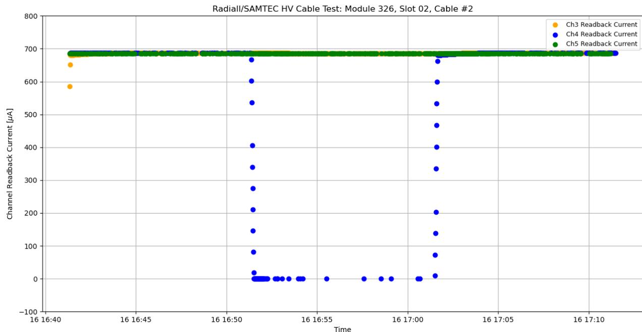
Channel 4 of cable #2 switching test done on CAEN A7030TN module #326
