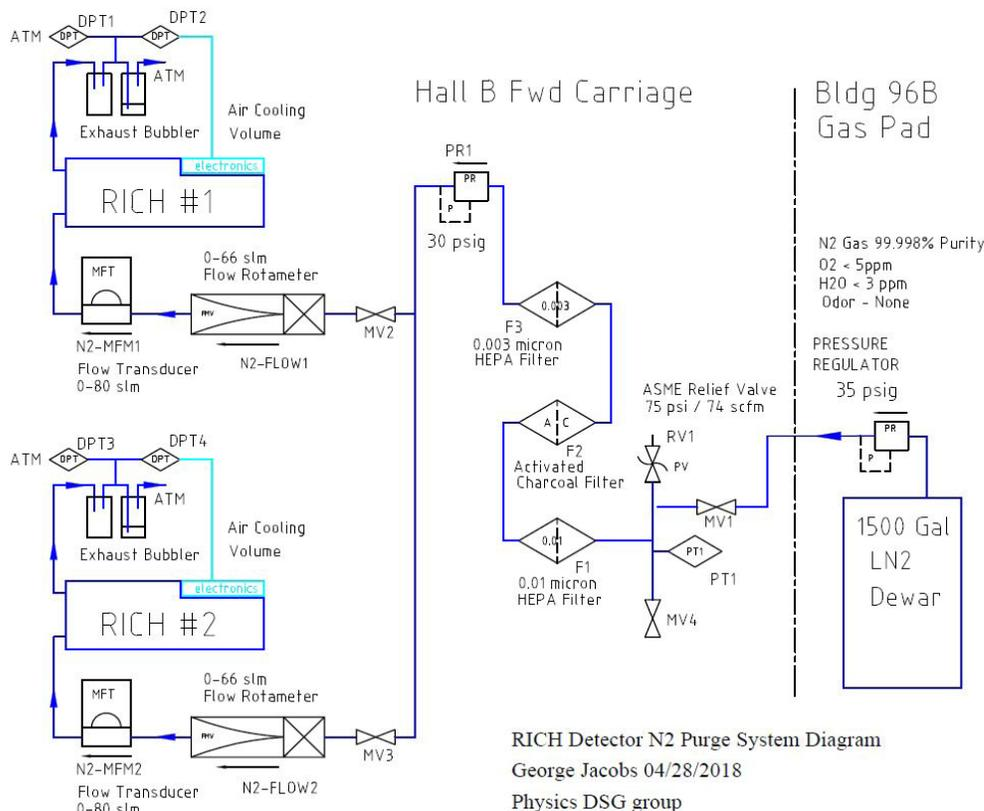
FIG. 1. Piping and instrumentation diagram of RICH nitrogen purge system.
