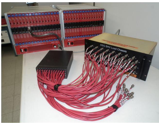
FIG. 1. A photograph of the test setup, showing the CAEN crate loaded with modules, black high voltage distribution load box, and load chassis.
