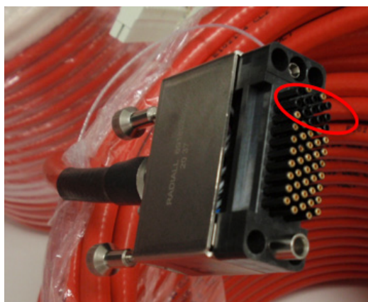
FIG. 2. Radial 52-pin connector; unused sockets circled in red.
