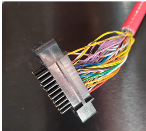
FIG. 3. Terminated wires in Radiall connector.
