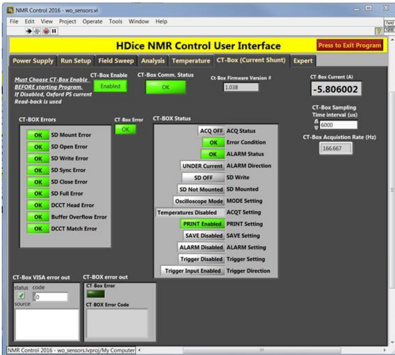
CT-BOX control and status readback tab in NMR program
