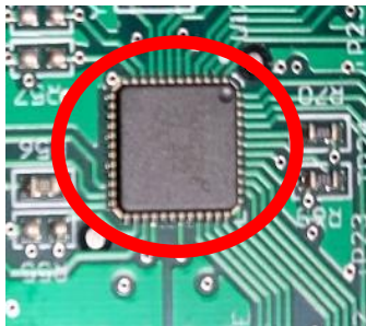
16-channel, 24-bit ADC on MSELV Chassis Sensor Readback board.
