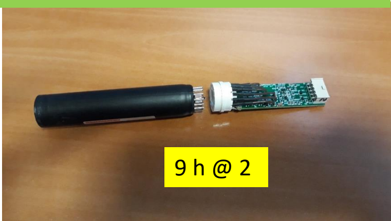
reflective sheets wrapping with tape (1080 crystals)
