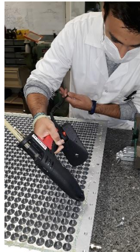
Gluing T° sensors wires on Reference plate
