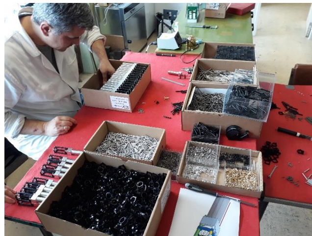
Assembling 1080 PMt support
