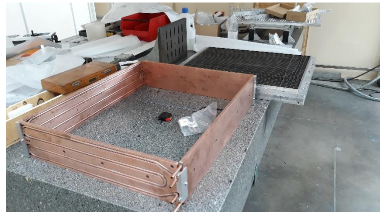
Pre-assembly cooling plates
