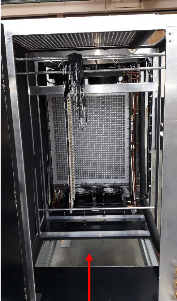
Remove the metal plate which is screwed on the bottom wood support (2 screws)
