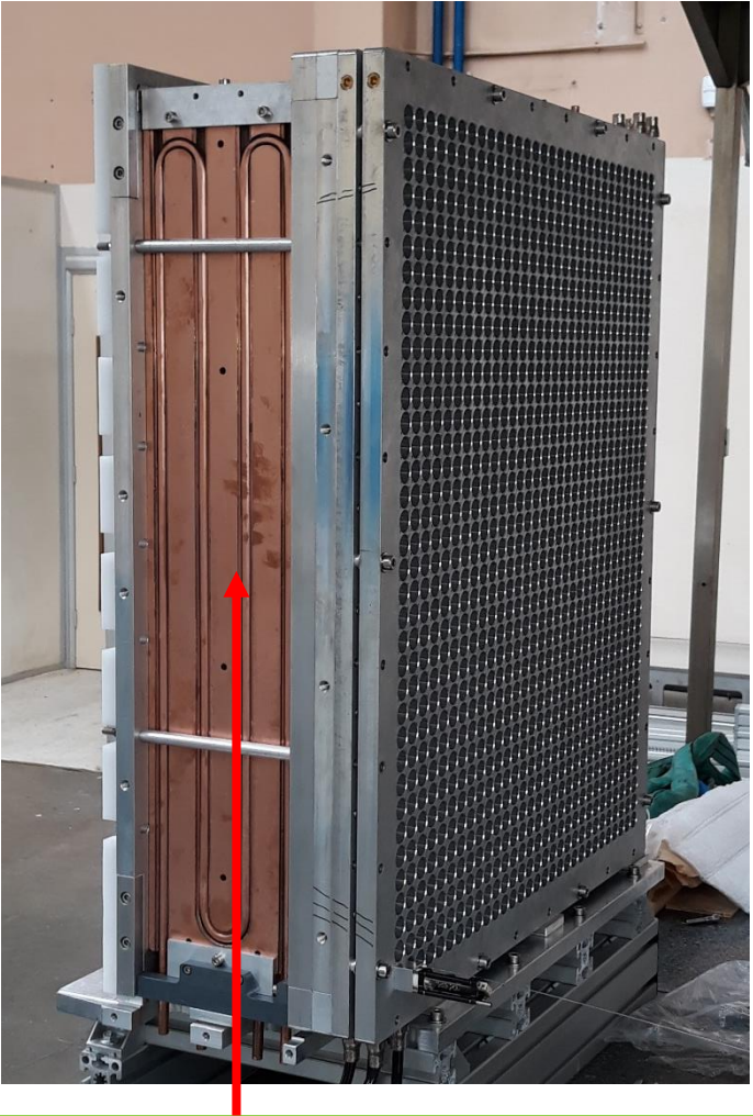
17 : remove the 4 Copper cooling plates
