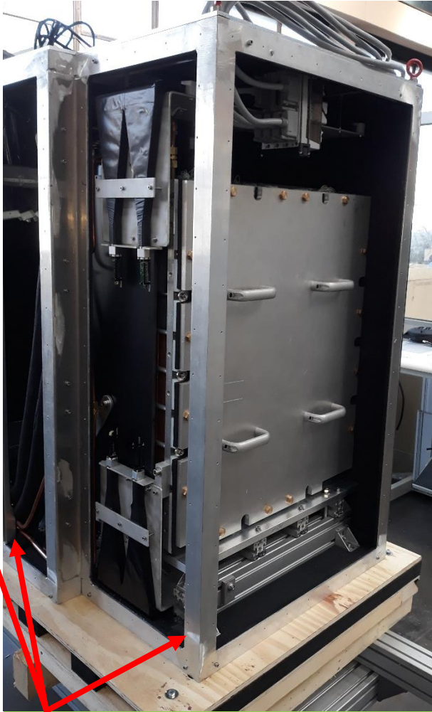
Remove the screws which maintain the Aluminum frame on the bottom wood support (6 screws)
