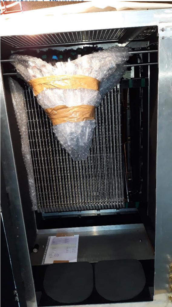
Remove the protection of anode cables
