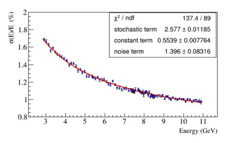
Preselected SICCAS crystals showed good performance due 12x12 prototype beam tests.
