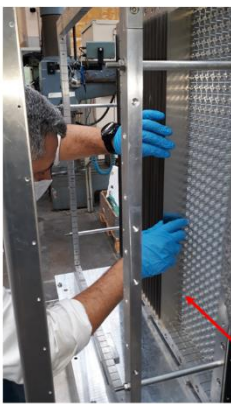
Slide the vertical mu metal plates (caution don't bend them ,very fragile)
