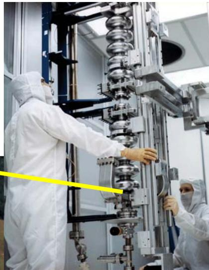
Superconducting radiofrequency (SRF) cavities undergo vertical testing.
