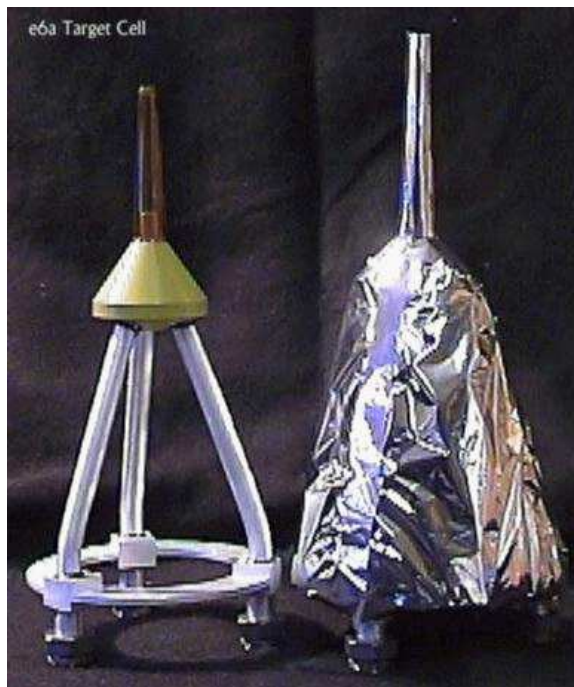
Figure 15: The E6 target cell with plumbing exposed (left) and with heat shields in place (right).
