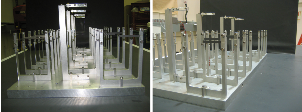
Figure 8: Left photograph: Front view of the target sections, where from left to right the production, empty, alignment, and optics sections can be seen. Note the alternating orientations of the carbon foils in the optics section – this allows the beam to pass through two different sets of 4 foils (with 14 cm spacing along the beam line), or all 8 foils (with 7 cm spacing). Right photograph: front-side perspective showing the layout of the target sections.
