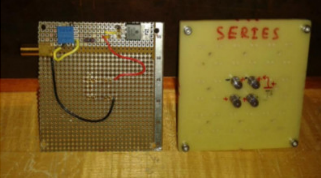
Figure 9: Partly assembled Infrared LED curing system.
