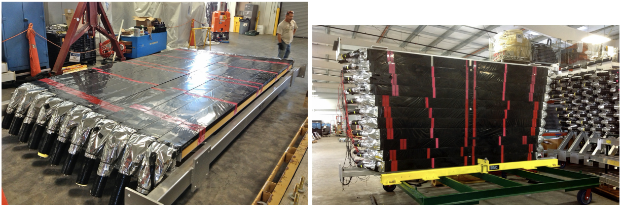
Figure 4: Left: One panel (11-bars) of the LAD detector lying flat on its frame; (right) Two panels of the LAD detector as stored on the storage cart in the ESB. Six panels of the LAD detector stored on the 2nd cart can be seen on the right side of the picture.
