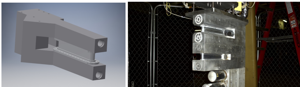
Figure 6: Left: CAD rendering of the LAD target cell, produced by D. Meekins; (right) photo HAPPEX target ladder, similar to what is designed for LAD.
