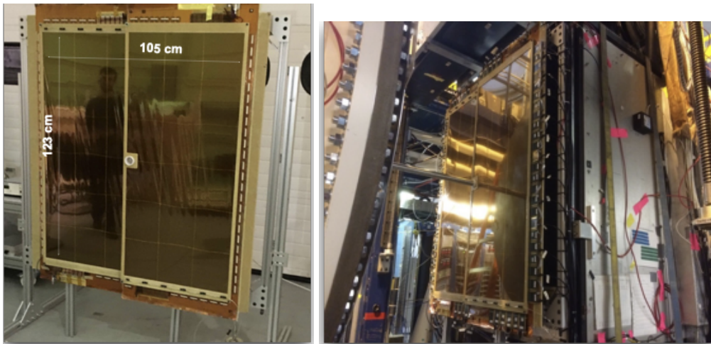
Figure 17: The PRad GEM chambers (left) and the GEM chambers mounted on the HyCal during the experiment (right).
