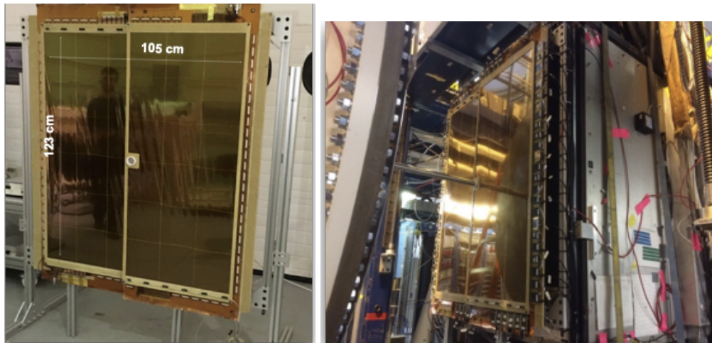
Figure 18: The PRad GEM chambers (left) and the GEM chambers mounted on the HyCal during the experiment (right).
