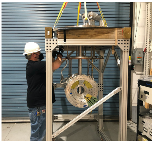
Figure 2: Left: JLab target group working on the newly arrived target magnet. Right: off-axis (vertical) field map at 5T with field uniformity < 100 ppm.
