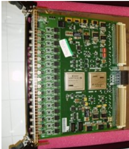
FIG. 18. FADC250 - Jlab 16 channel VME/VXS based 250Msp/s Flash ADC digitizer
