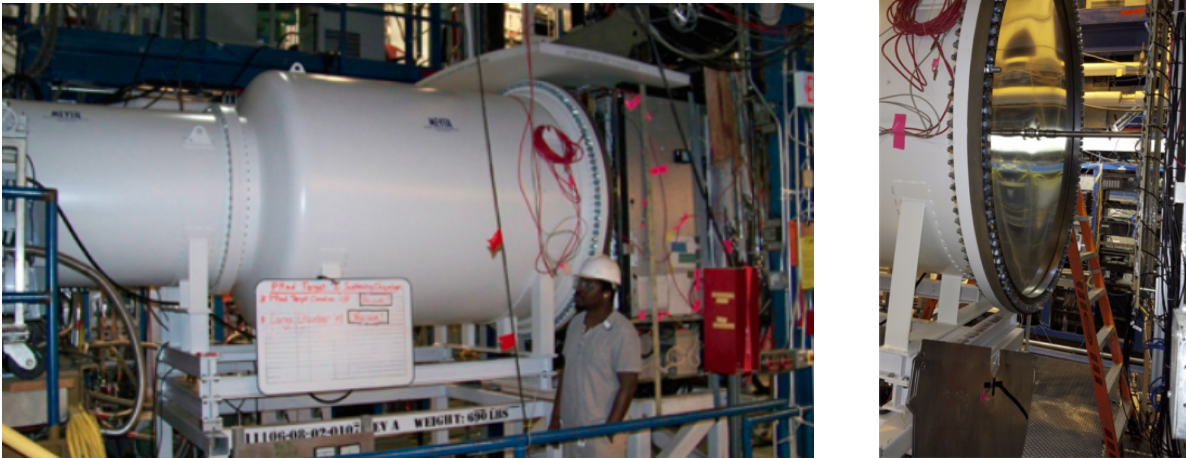
Figure 17: A photograph of the \sim 5 m long, two stage vacuum chamber used during the PRad experiment (left, please disregard the date on the photograph). A photograph of the 1.7 m diameter thin window at one end of the vacuum chamber (right). Here the GEM and HyCal have been moved downstream for technical service.
