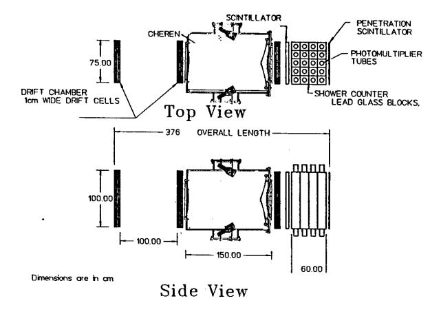
Fig. (5). The detector stack proposed for the HMS spectrometer used in the coincidence experiment. This arrangement is the same as described in the CEBAF Conceptual Design Report.
