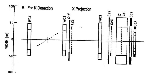
Fig. (6). The detector stack proposed for the SOS spectrometer used in the coincidence experiment. This compliment of subsystems is the same as described in the CEBAF Conceptual Design Report.
