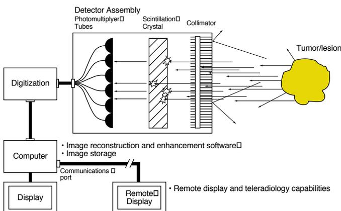
Simplified schematic of imaging system
