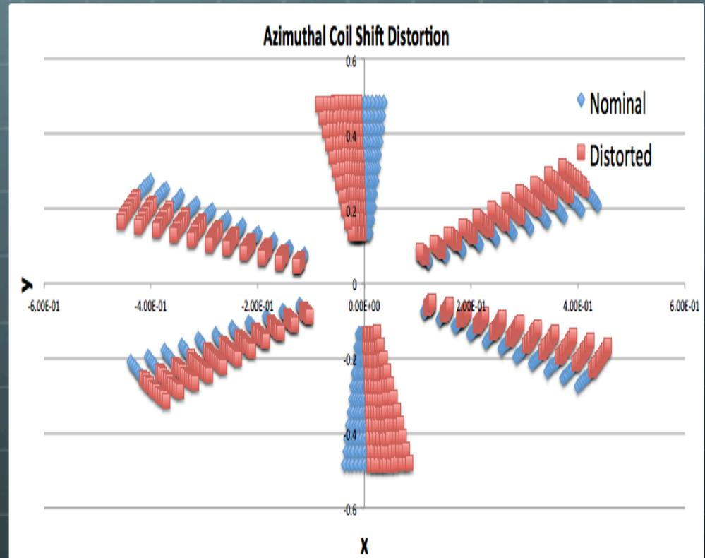
Fig. 3. An example of a possible coil displacement, a shift in azimuth
