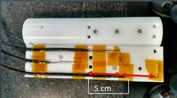
Fig. 8. The inside of the Hall probe
