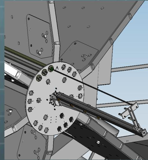
Fig. 7. Visual model of the Hall probe being pushed by a motor along the beam axis inside a non-magnetic Carbon tube
