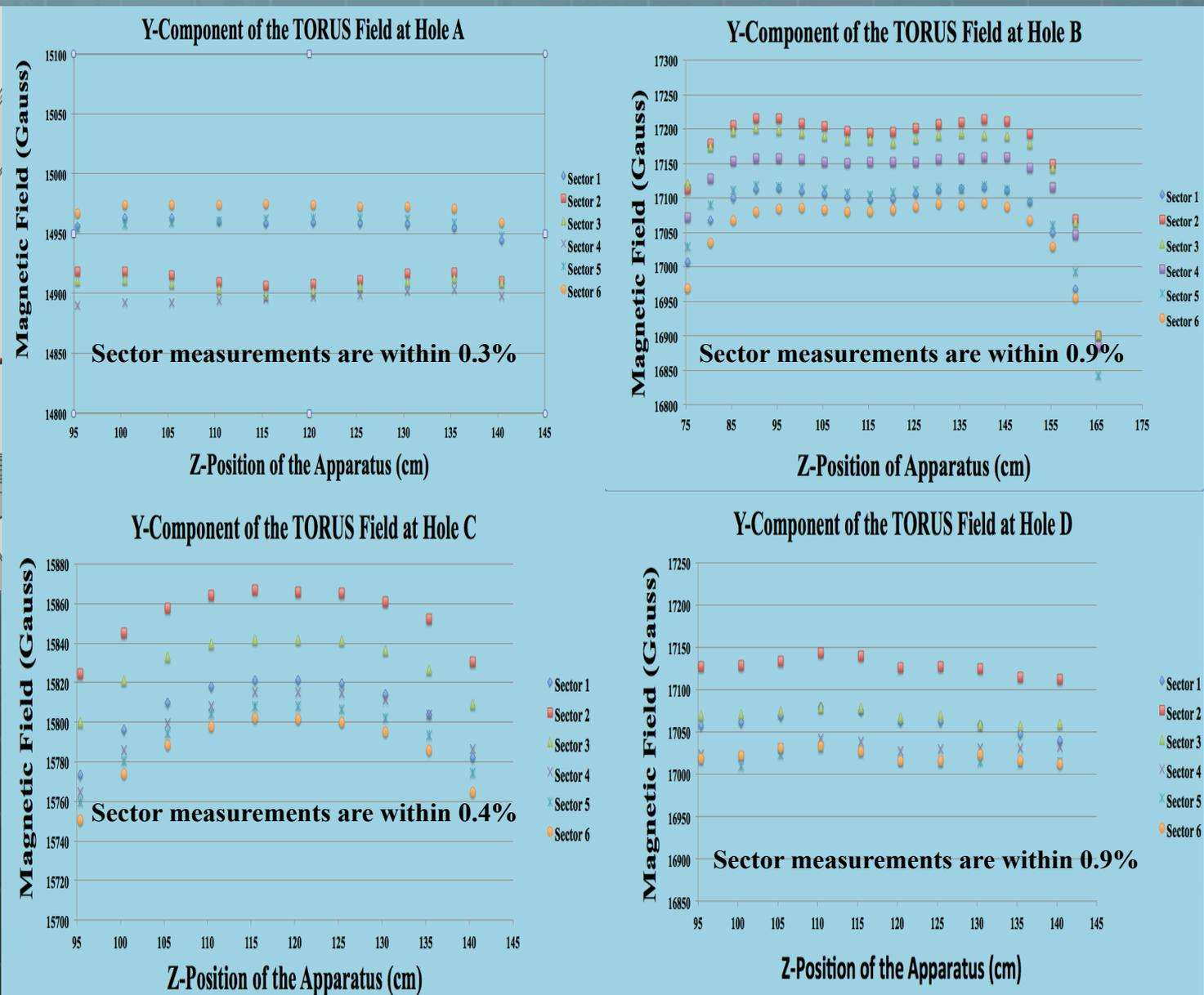
Fig. 10. Large component of the TORUS field at Holes A-D as measured in all six sectors.
