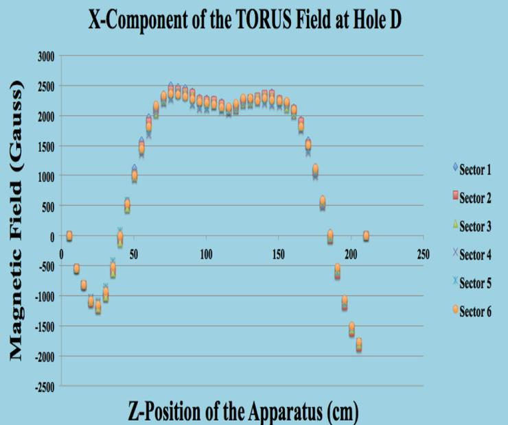
Fig. 11. X-component of the TORUS field at Holes A-D in Sectors 1-6.
