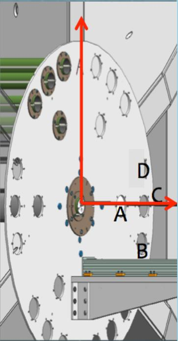
Holes A and C, which radially divide each sector should see no magnetic field. Any field can be an indication of a rotating reference frame
