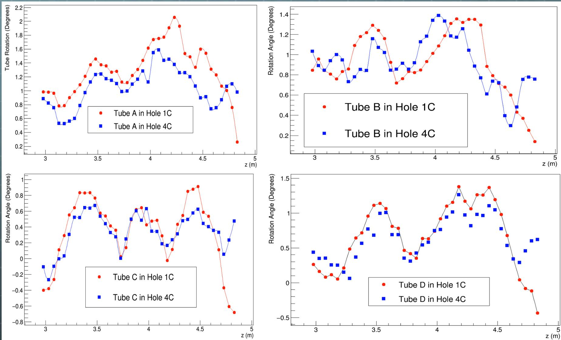
Fig. 13. Effect of tube on the rotation of the Hall probes.
