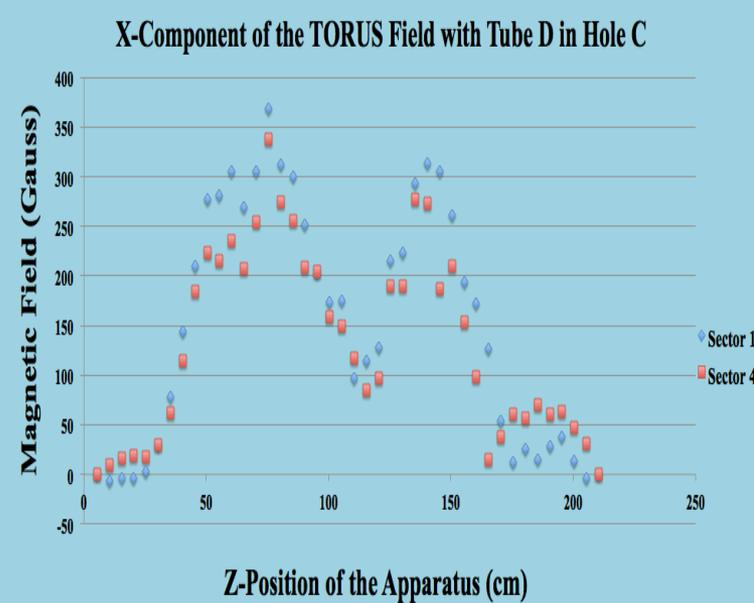
Fig. 12. X-component of the TORUS field at Hole C using different non-magnetic tubes to test for non-field effects to data
