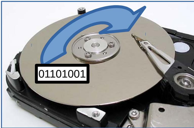
7200 RPMs => about 4 ms on average for the disk to spin to the necessary position to start reading the data.
