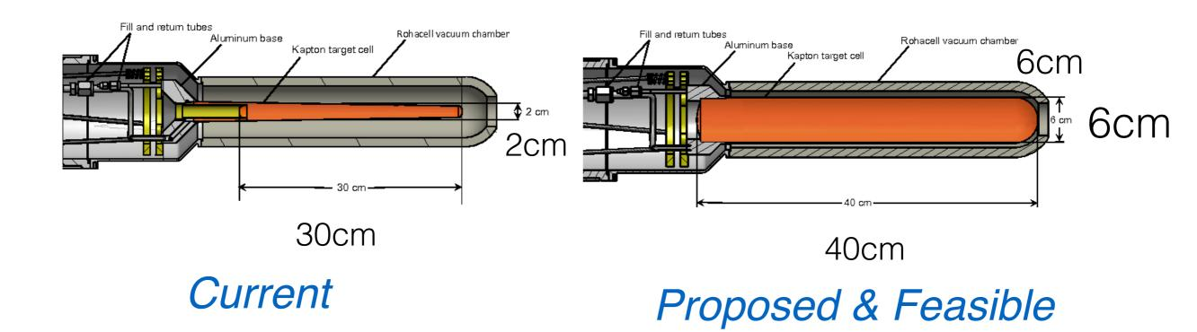
Longer and thicker target needed to enhance production rate
