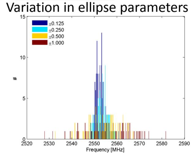
Loosened machining tolerances increase relative cavity-to-cavity HOM frequency spread (good!)
