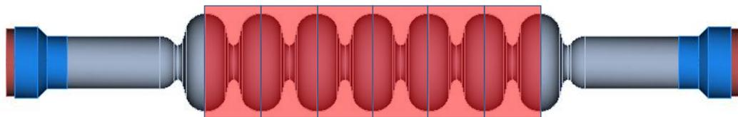
Seven-Cell Cavity Optimization for Cornell's Energy Recovery Linac
