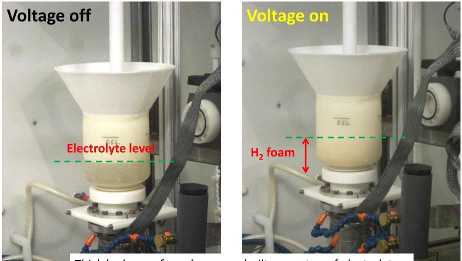
Thick hydrogen foam layer was built up on top of electrolyte during VEP voltage on so far.
