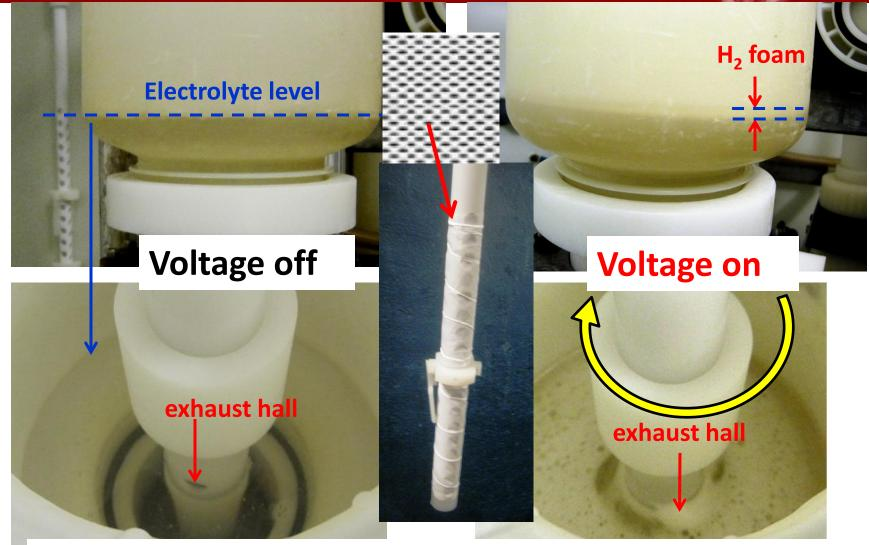
Cathode bag successfully guided hydrogen and reduced hydrogen foam layer.
