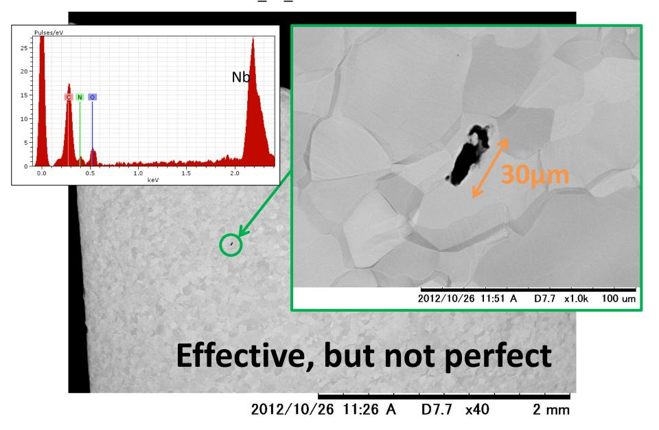
Ultrasonic cleansing with degreaser (FM20)
