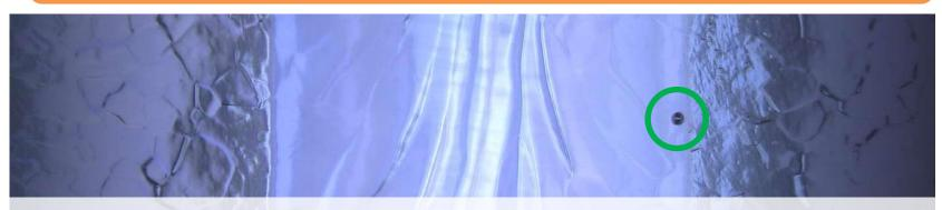
On and around electron beam welding (EBW) seams, however, defects are often found.
