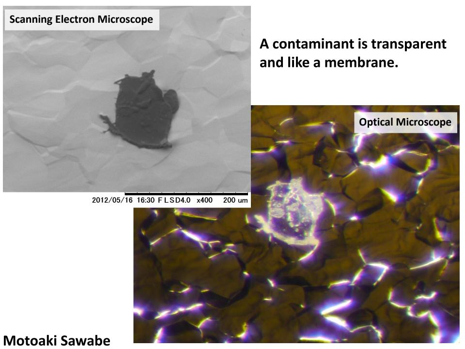
EDX analysis indicates the contaminants contain "carbon", "oxygen" and sometimes "nitrogen".
