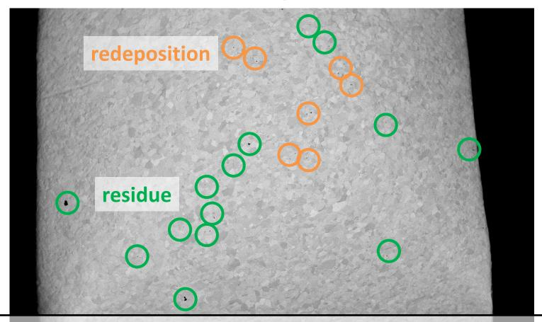
We can not remove "carbon including contaminants" by ultrasonic cleansing with acetone.
