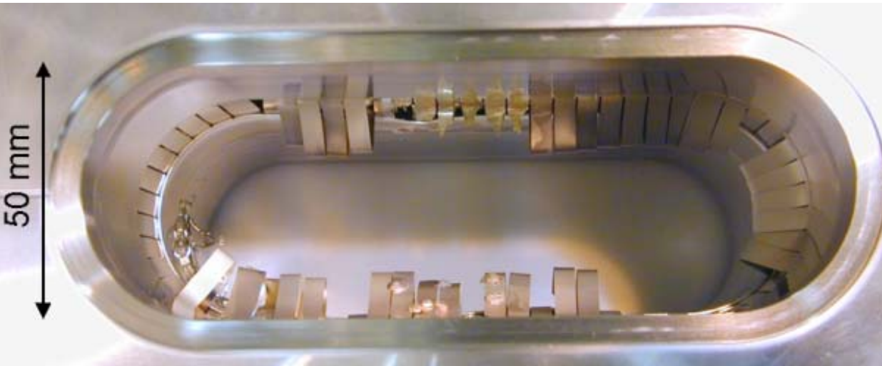
Damaged RF shield fingers
