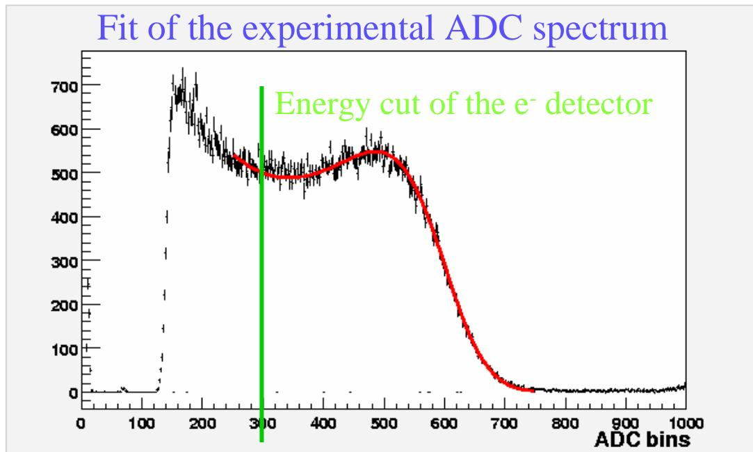
$$\frac{d\sigma(ADC)}{dADC} = \int_0^{k_{\max}} \frac{d\sigma_0(k)}{dk} g(ADC, k) dk$$
