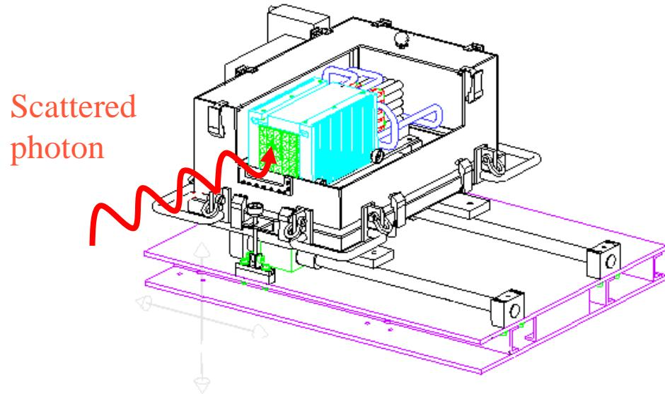
25  $\text{PbWO}_4$  scintillators ( $2 \times 2 \times 23 \text{ cm}^3$ )
