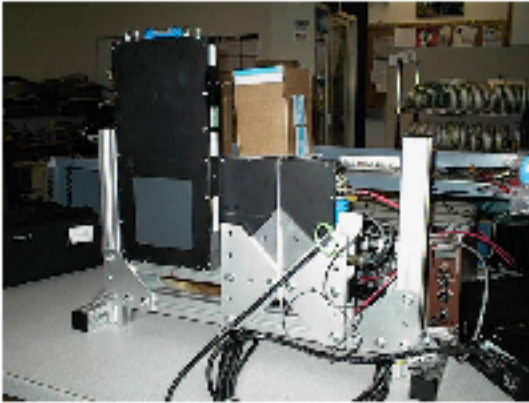
Figure 25: The PrimEx photon beam position detector.
