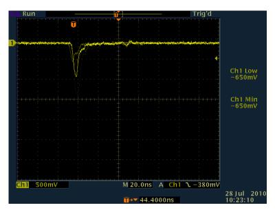
The pictures both above and below this caption are examples of signals received by the Digital TekTronix Oscilloscope that I used to test each PMT output. The signal shown is caused by the incidence of cosmic rays on the scintillating paddles of the Veto Detector. These signals are what I
