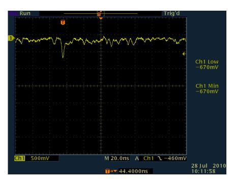
This image from the oscilloscope is a result of light leakage into the protective black plastic covering of the paddle.
