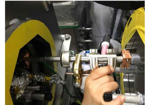
[Lip-seal alignment and tack welding]
