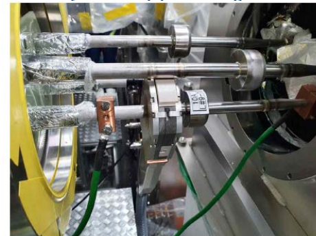
[Auto welding of the pipe]
