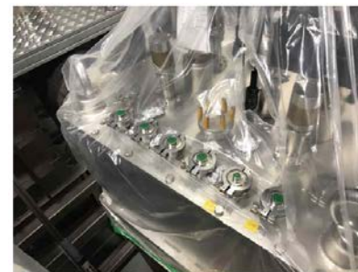
[Short 4-wire temperature sensors to protect current leak]
