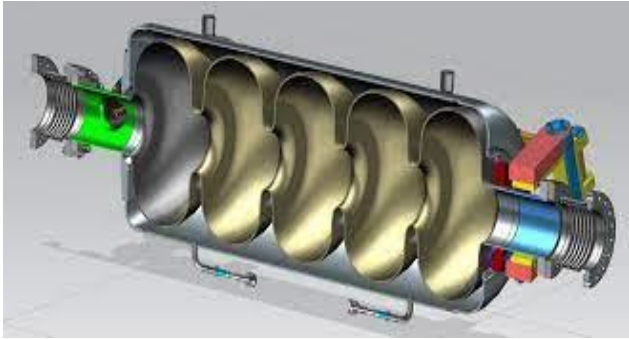
Half of the multicell cavity showing inner view
