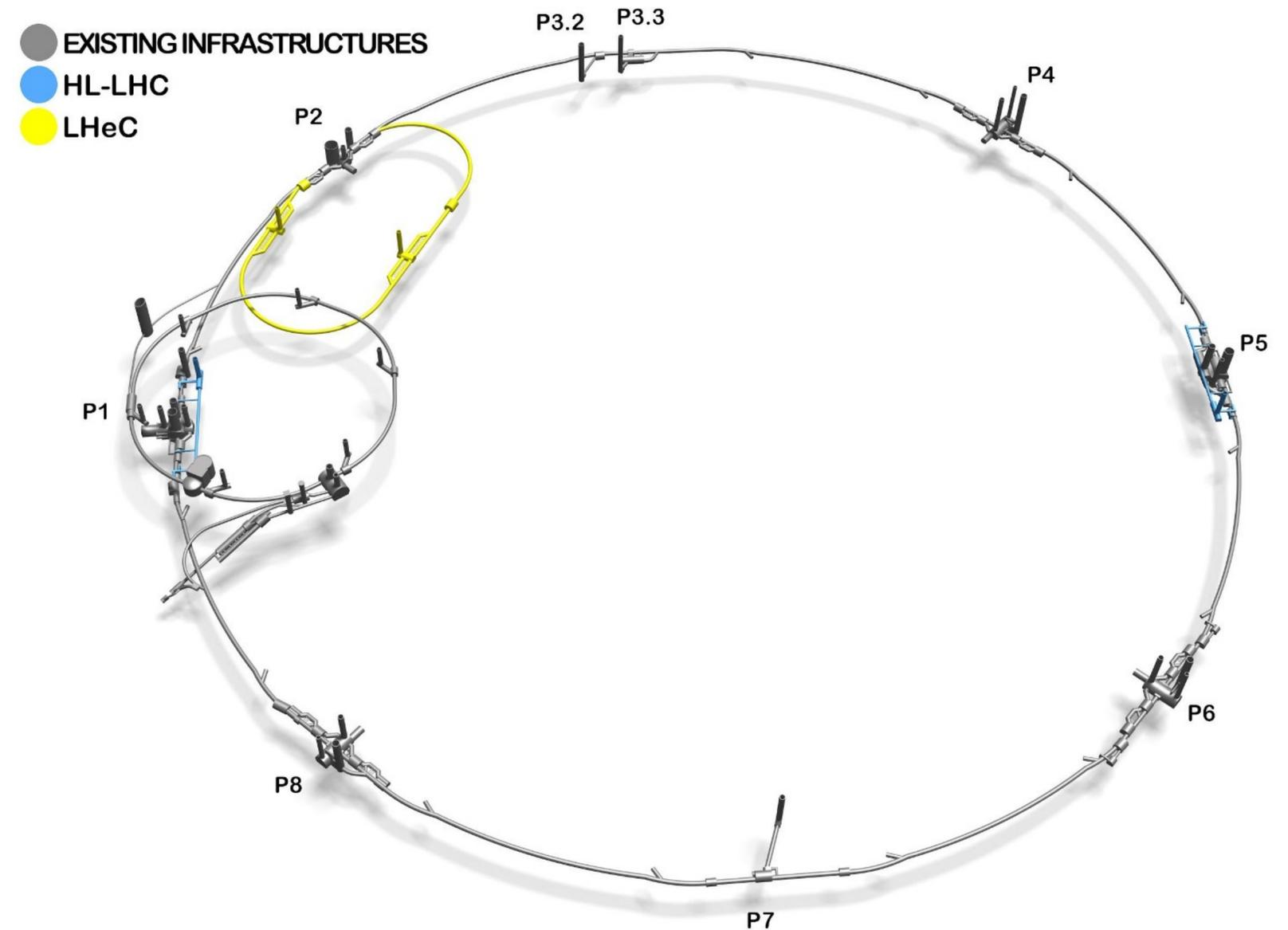
High power electron beam based on three-turn ERL racetrack utilising 100 MW electrical power consumption as a result of the high energy recovery efficiency. ERL circumference equivalent to one-third of the LHC. The ERL could be realised in staged phases.
