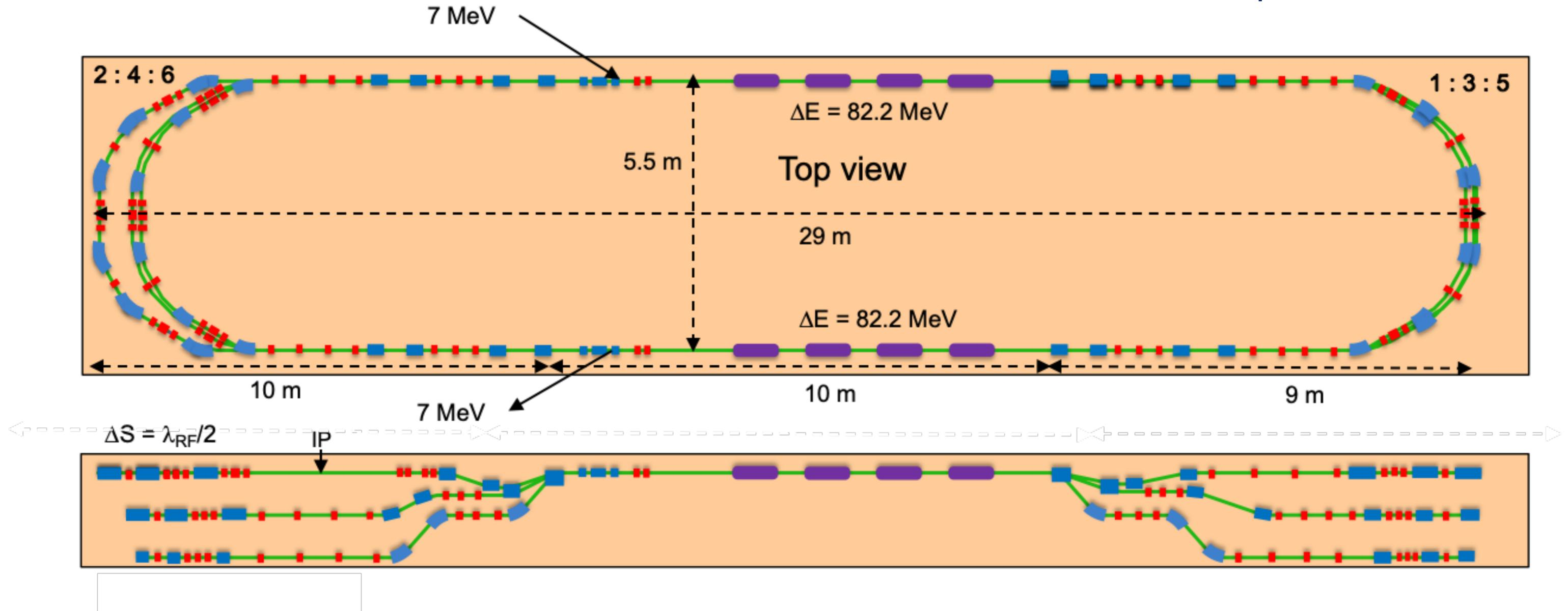
Denis Reynet (Département Mécanique, IJCLab) proposed to **flip the lattice vertically** to have an easier access to the IPs
