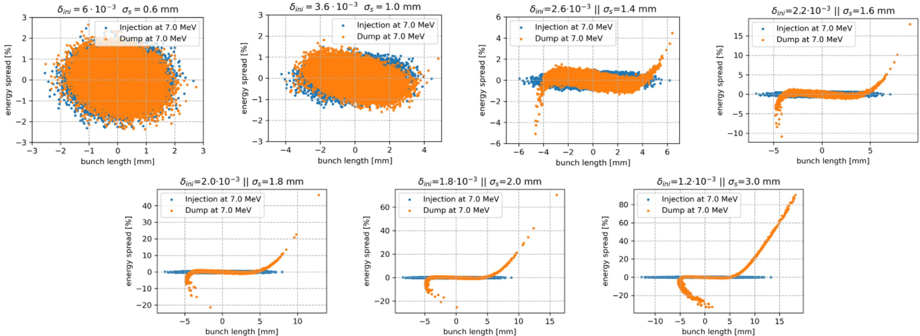
A hook shape forms and bunch elongation is visible as the initial bunch length increases. A longitudinal matching can mitigate the bunch elongation.
