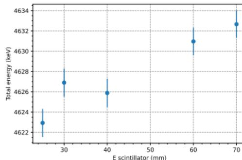
Energy deposited in 51 mm diameter E scintillator vs length.
