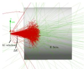
5 MeV beam through Al = 200  $\mu\text{m}$ ,
