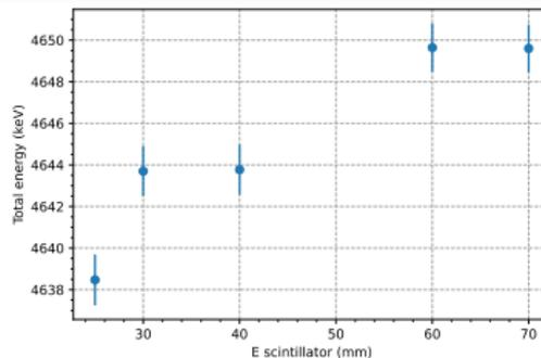
Energy deposited in 76 mm diameter E scintillator vs length.
