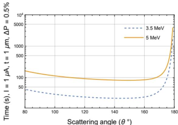
Measurement time required for corresponding angles.
