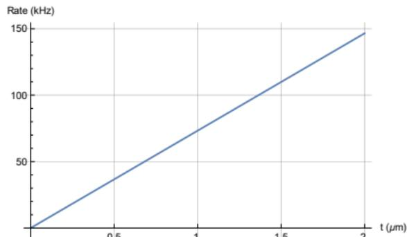
Total scattering rate for  $I = 150 \mu\text{A}$ ,  $E = 5 \text{ MeV}$ ,  $\Delta\Omega = 0.23 \text{ mSr}$
