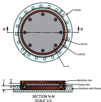
Design of the beam dump. Dimensions are in mm.
