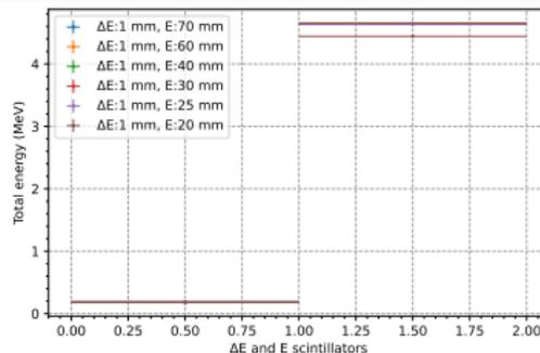
Energy deposited in 76 mm diameter E scintillators.
