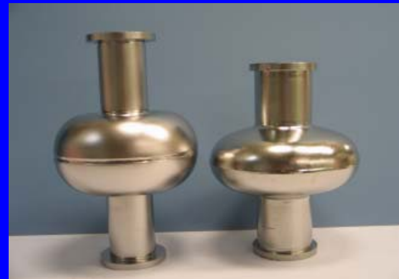
Left: 60 mm aperture reentrant cavity; Right: 70 mm aperture TESLA cavity.
