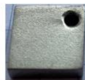
Conventional vapor-diffused Nb 3 Sn
