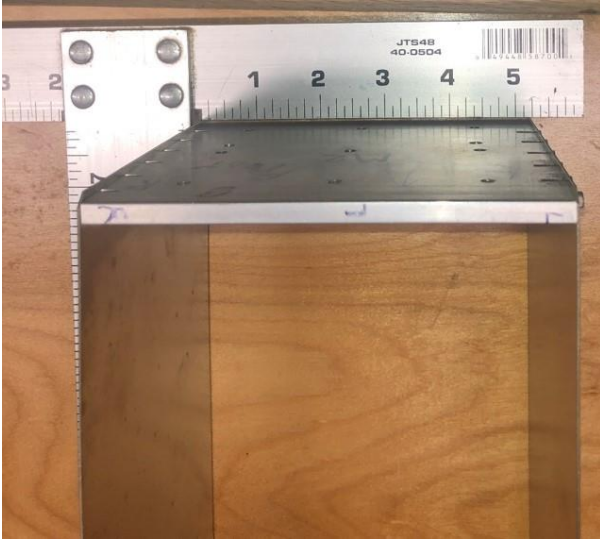
Figure 2. Supermodule frame top view, width is just over 5".
