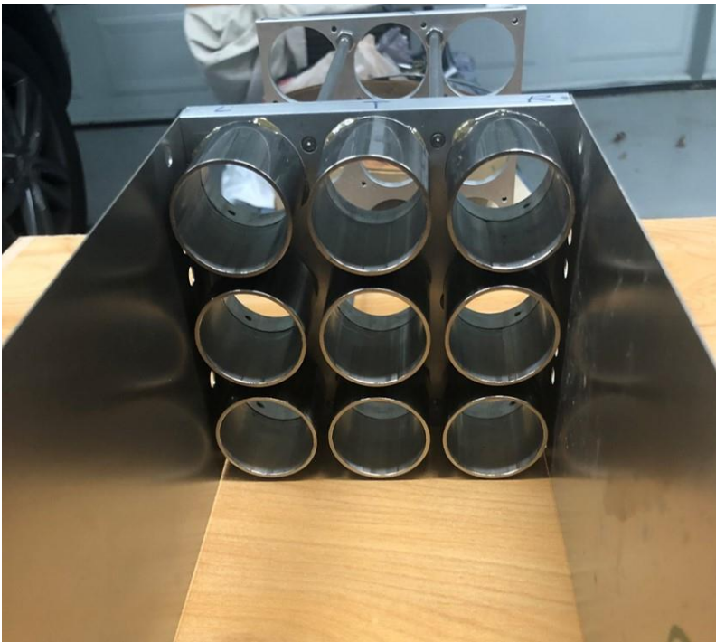
Figure 3. Inside view of the base direction. These bases should be checked for planarity across the top surface and misalignment with the base flange
