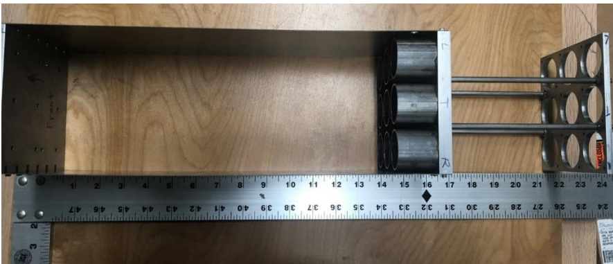
Figure 1 Supermodule frame_top view. The frame is about 2' long.
