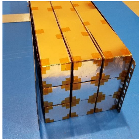
Figure 4. Flange 1 end of lead-glass (9 pieces) prior to clamping
