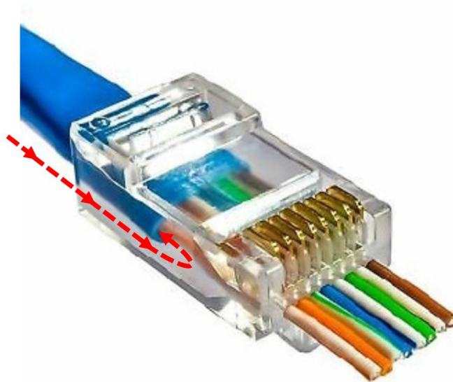
Dashed, red arrow shows path of suspected leak from one side of feedthrough to other
